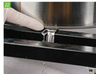
22 Install the barrel body on the base, pay attention to contact the barrel body with the grounding chain
