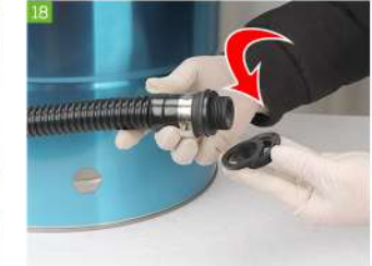
18 Rotate the plastic nut at one end of the drain pipe thread to open, there are 2 pieces of rubber in it, take out one piece
