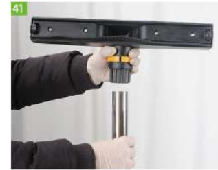
Install the vacuum cleaner and the squeegee on the other end of the steel pipe, and then screw them together to increase the friction to make them tighter.
