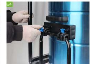
24 Press down the 2 buttons on the side to fasten the barrel body and the base
