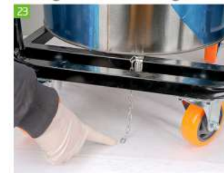
23 Note that the grounding chain needs to be in contact with the ground to ensure the export of static electricity
