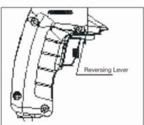
A CAUTION of rotation until the tool Do not change direction comes to a complete stop. Shifting during rotation of the chuck can cause damage to the tool.
