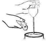
Hold the test cup up and measure the time in seconds until the liquid empties out. This time is referred to below as Runout Time.
