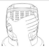
Remove the dirty filters and replace with new ones.
